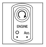
Your vehicle has an electronic keyless ignition with pushbutton start.
